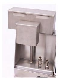
Water Baffle option filters the smoke from the exhaust through a water bath which can eliminate the need for a vent hood to operate.
